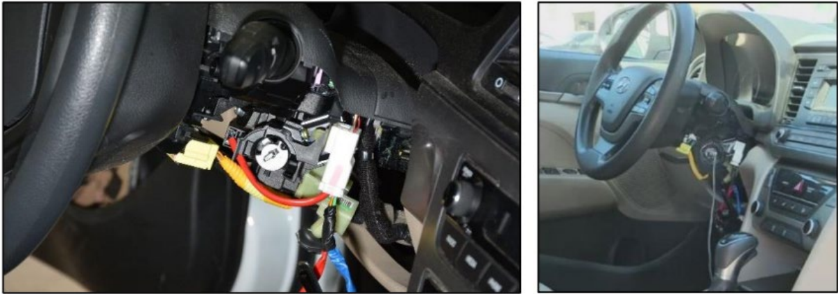
Example photos of a punched ignition column and USB charging cable used to start a vehicle.
